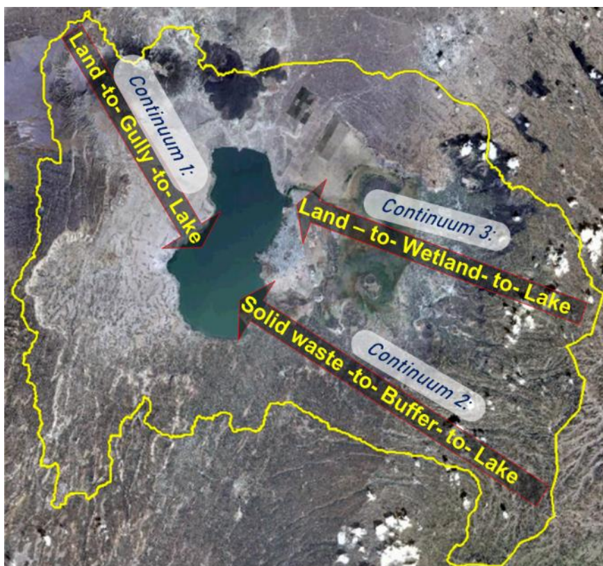
Figure 7. Typical source-to-lake continuum characterizing the sediment flow in Lake Hawassa sub-basin
