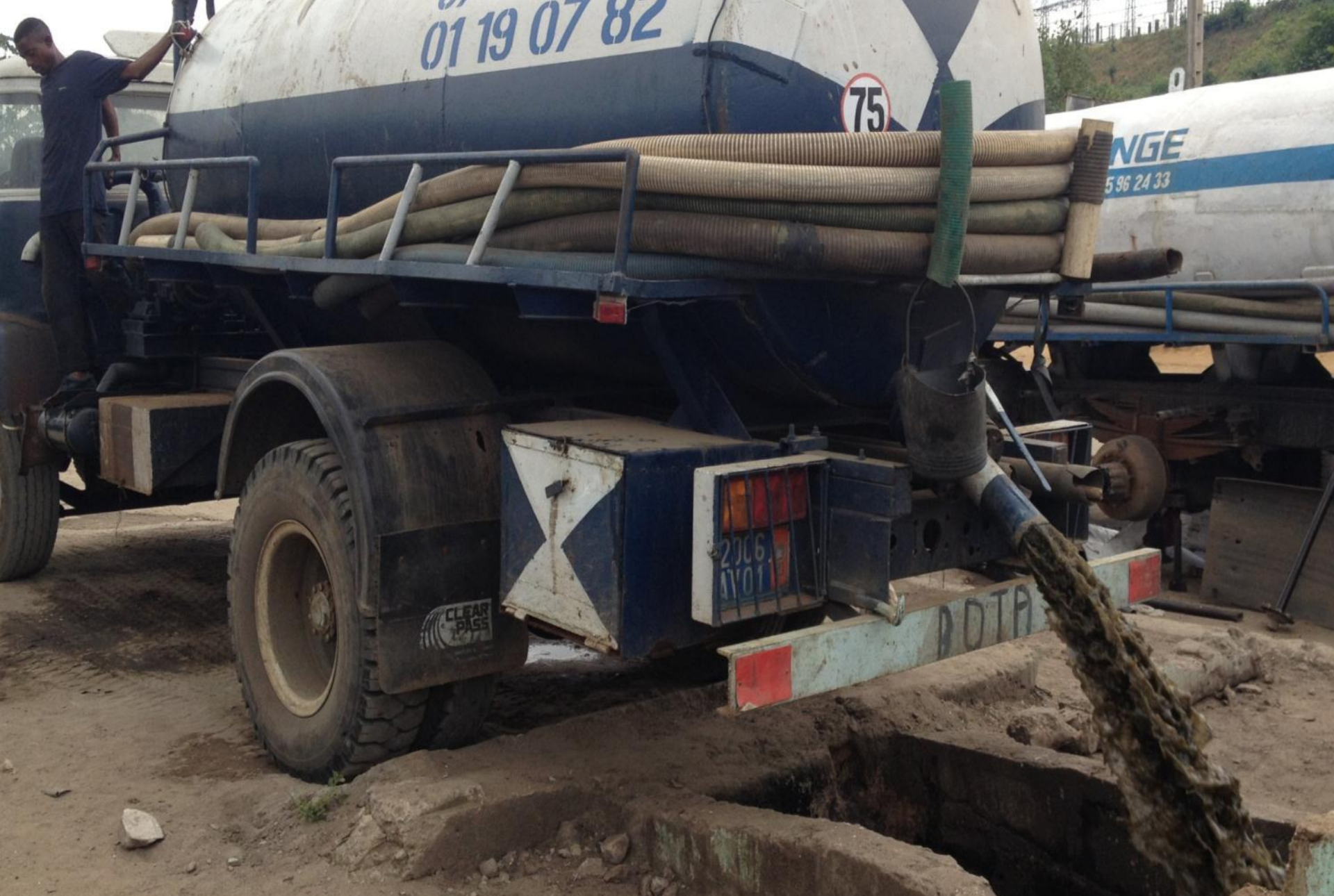
Current Solution #2: Septic Trucks -Step 1: Waste is collected and emptied at designated dump site
